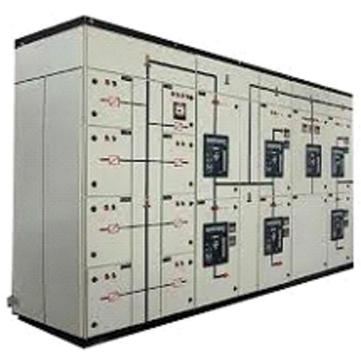
It consists of feeders for motors and blowers. Feeders are designed according to the motor rating. In most of the MCCs, auto/manual provision will be there. With manual provision motors can be operated manually. In auto provision external signal is required to start the motor. The signal is given by the control panel. Indicators for the motor operation also will be present in control panel.
