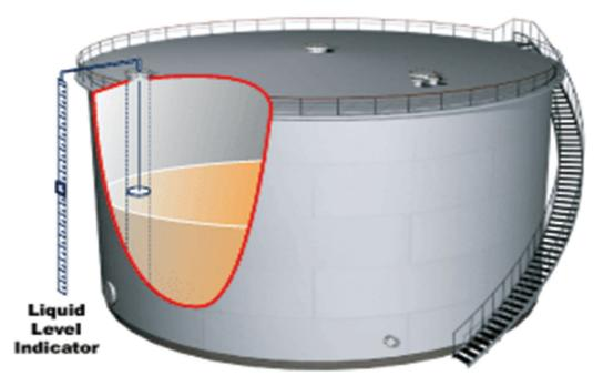
Scales are marked in cms, in reverse order, zero level marking on top and total tank height in cms at bottom. PP construction for acid application is also available. Indicators are manufactured in different operating ranges as per tank heights for both underground & overhead tanks in either vertical or horizontal tanks.
