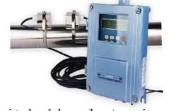
Transmitter and receivers roles are constantly switched by electronics. Ultrasonic pulses travelling in the direction of the flow, travel path between transducer in a shorter period of time than pulses travelling against the flow. This is because the flow speeds up pulses travelling downstream but slows down pulses travelling upstream.
